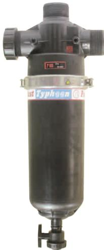
The filter has 1 inlet and 2 alternative outlets depending on requirement. Available with male thread 2" - 3" (SSS) or VICTAULIC Φ63-2", Φ90-3" (VVS) for battery systems.
